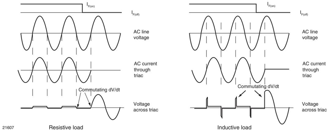
Fig. 12 - Waveforms of Resistive and Inductive Loads
