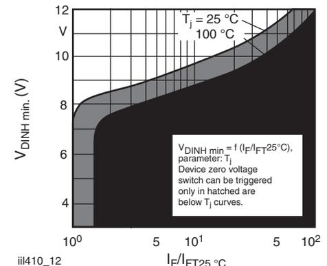
Fig. 10 - Typical Static Inhibit Voltage Limit
