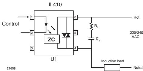
Fig. 15 - Basic Direct Load Driving Circuit
