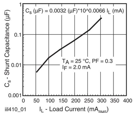
Fig. 13 - Shunt Capacitance vs. Load Current
