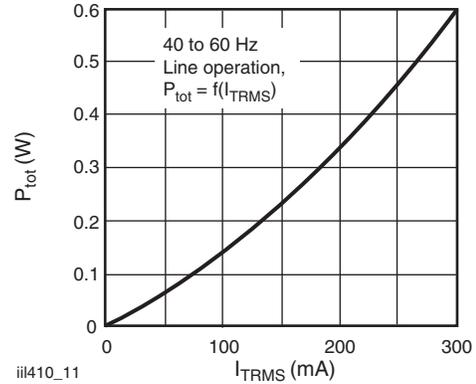
Fig. 9 - Power Dissipation 40 Hz to 60 Hz Line Operation
