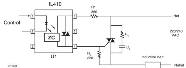
Fig. 16 - Basic Power Triac Driver Circuit
