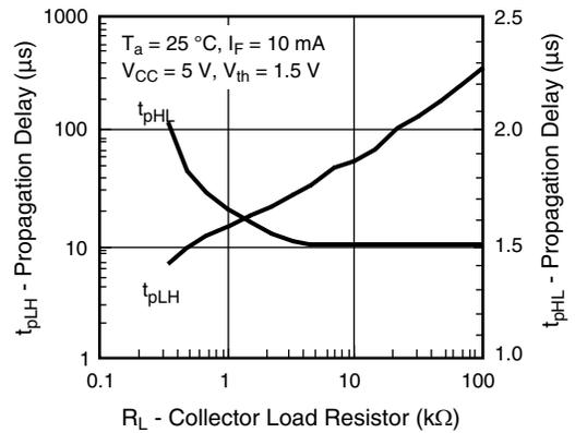
Fig. 12 - Propagation Delay vs. Collector Load Resistor
