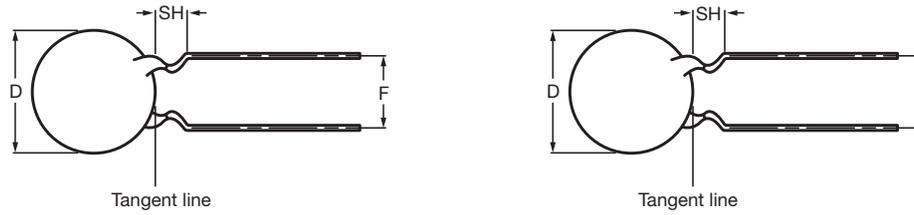
Capacitors with 5 mm (0.20") and 7.5 mm (0.30") lead spacing
