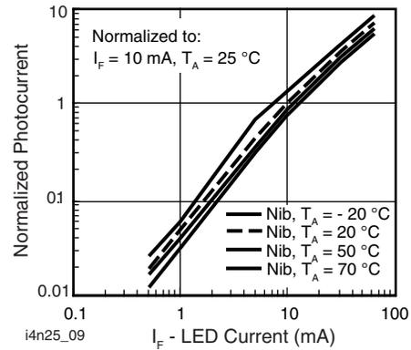
Fig. 9 - Normalized Photocurrent vs.  $I_F$  and Temperature
