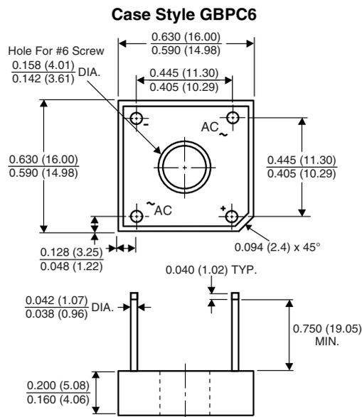
Polarity shown on side of case: Positive lead by beveled corner
