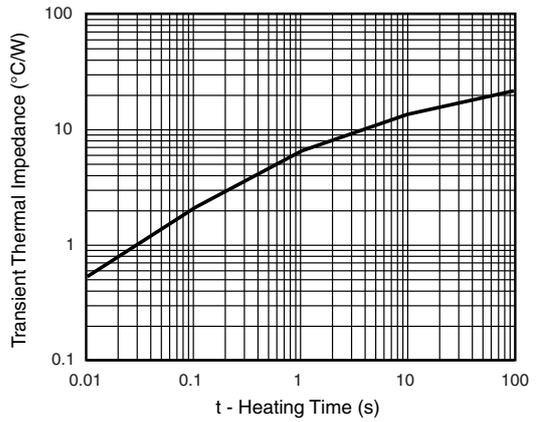
Fig. 6 - Typical Transient Thermal Impedance Per Diode
