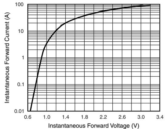
Fig. 3 - Typical Forward Characteristics Per Diode
