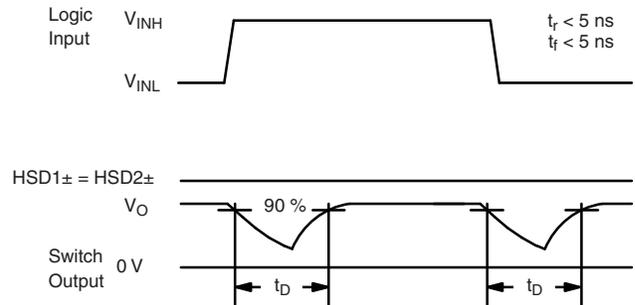
Fig. 2 - Break-Before-Make Interval
