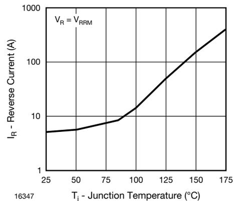
Fig. 4 - Reverse Current vs. Junction Temperature ( $^{\circ}\text{C}$ )
