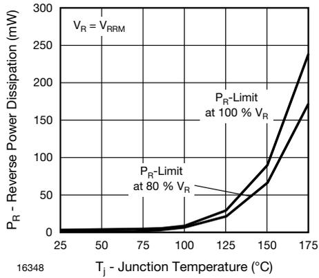
Fig. 5 - Max. Reverse Power Dissipation vs. Junction Temperature
