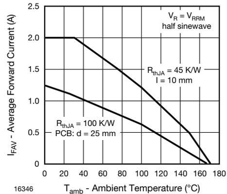
Fig. 3 - Max. Average Forward Current vs. Ambient Temperature
