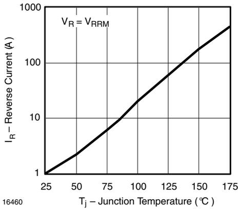
Fig. 5 - Reverse Current vs. Junction Temperature
