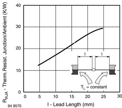
Fig. 1 - Max. Thermal Resistance vs. Lead Length
