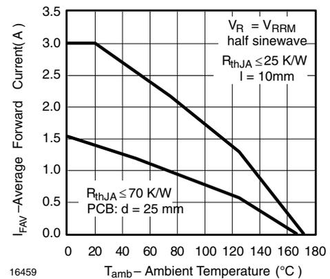
Fig. 4 - Max. Average Forward Current vs. Junction Temperature
