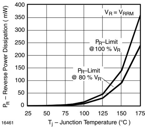
Fig. 6 - Max. Reverse Power Dissipation vs. Junction Temperature
