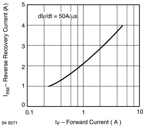
Fig. 2 - Typ. Reverse Recovery Current vs. Forward Voltage
