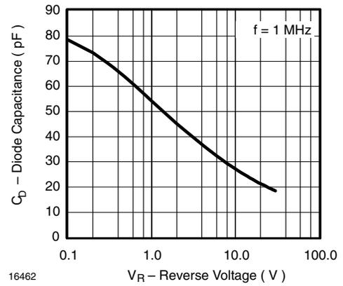
Fig. 7 - Diode Capacitance vs. Reverse Voltage
