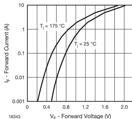
Fig. 4 - Forward Current vs. Forward Voltage
