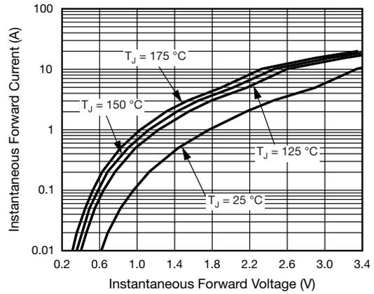
Fig. 4 - Typical Instantaneous Forward Voltage Characteristics
