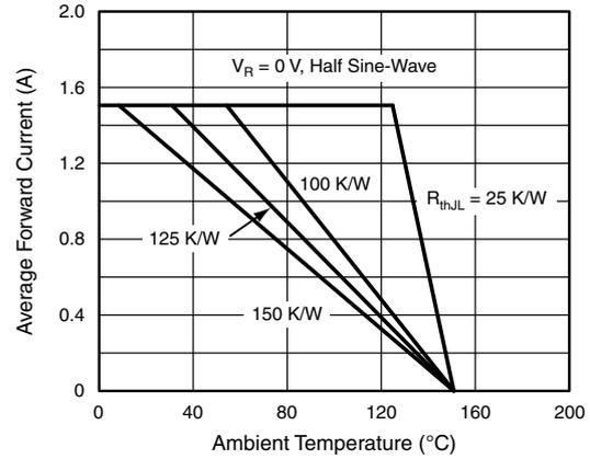
Fig. 4 - Max. Average Forward Current vs. Ambient Temperature
