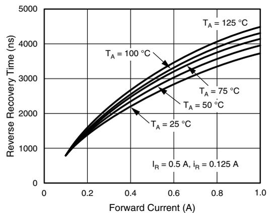
Fig. 6 - Reverse Recovery Time vs. Forward Current
