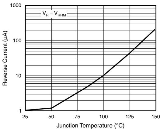
Fig. 3 - Reverse Current vs. Junction Temperature
