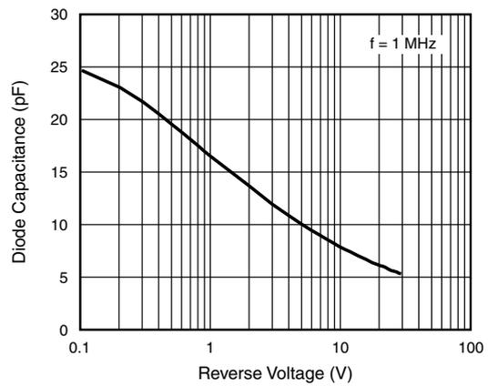
Fig. 5 - Diode Capacitance vs. Reverse Voltage
