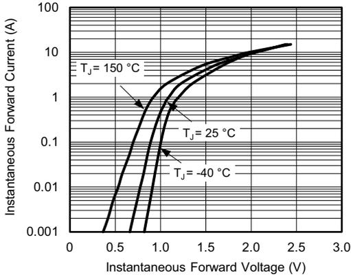
Fig. 1 - Forward Current vs. Forward Voltage
