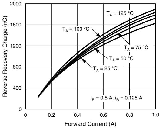
Fig. 7 - Reverse Recovery Charge vs. Forward Current
