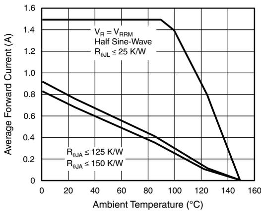
Fig. 2 - Max. Average Forward Current vs. Ambient Temperature
