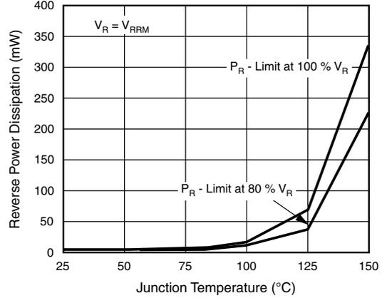
Fig. 4 - Max. Reverse Power Dissipation vs. Junction Temperature
