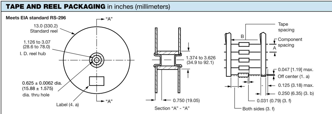
**STANDARD PACKAGING QUANTITY AND DIMENSIONS** in inches (millimeters)
