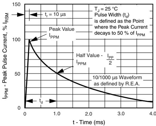
Fig. 3 - Pulse Waveform
