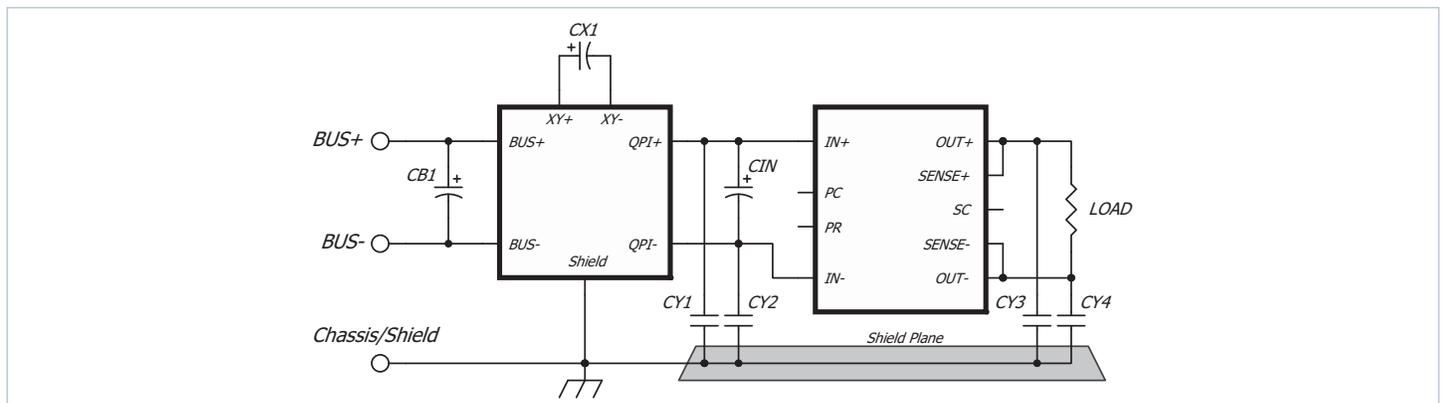
Figure 2 — Typical QPI-21 circuit with a Vicor brick converter. Optional X (CX1) filter capacitor shown.<sup>[b]</sup>
