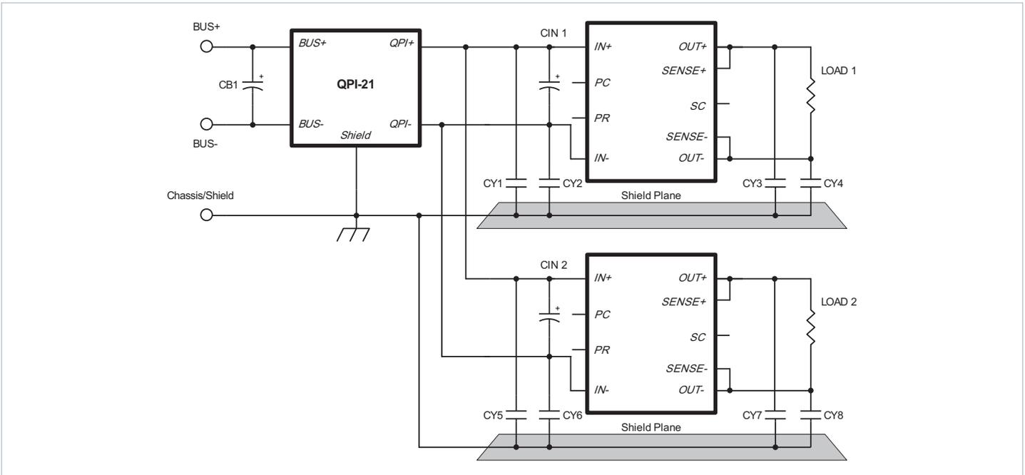
**Figure 15** — The QPI-21 filtering dual supplies.<sup>[e]</sup>
