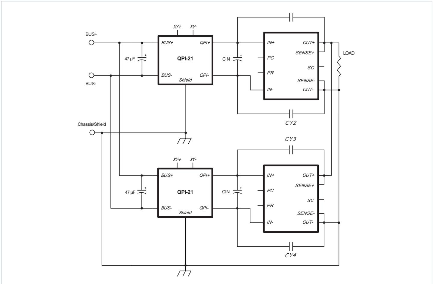
**Figure 16** — Dual QPI-21's filtering paralleled converters feeding a common load.<sup>[e]</sup>
