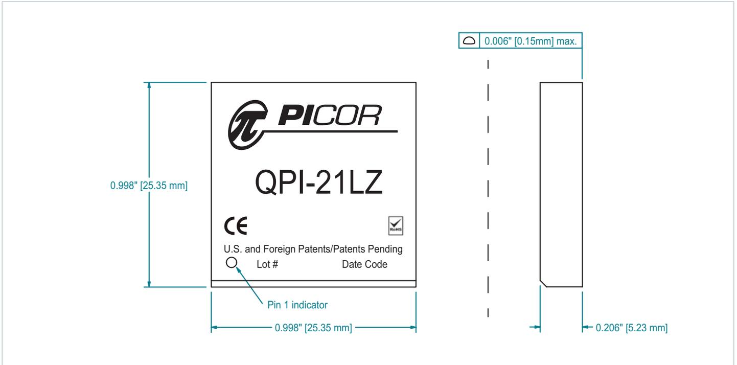
Figure 20 — Lidded Package Dimensions, tolerance of  $\pm 0.004$ "
