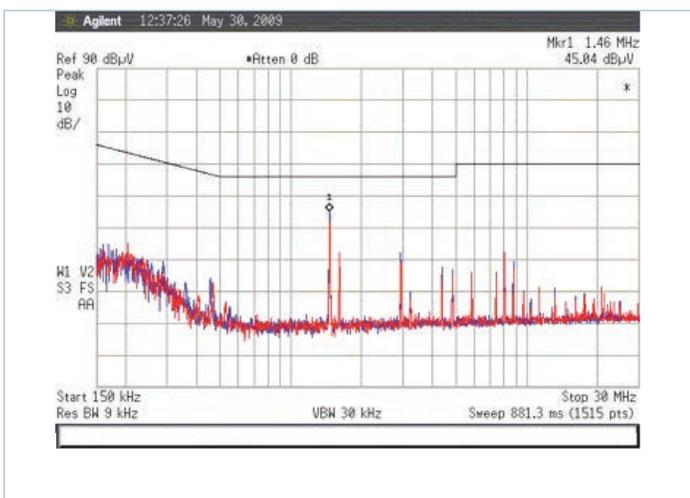
Figure 5 — VTM V048F240T012-CB with 172W output load
