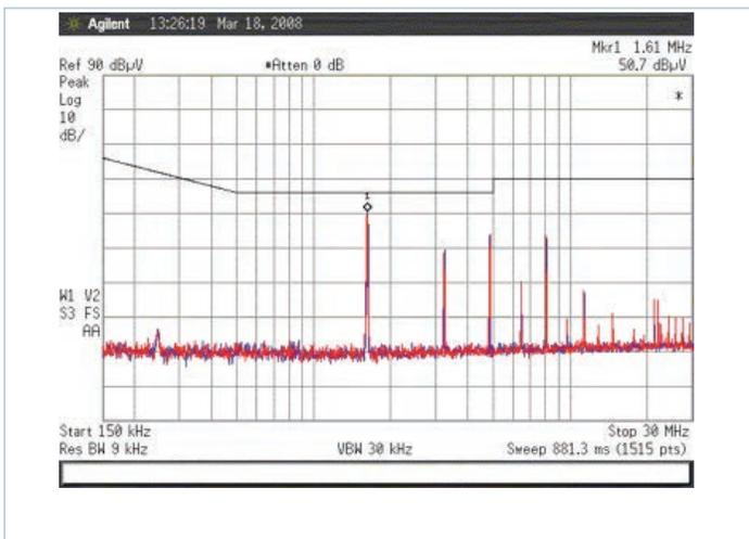
Figure 9 — BCM B048F240T30-EB with 172W load
