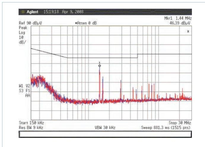
Figure 4 — VTM V048F120T025-CB with 180W load
