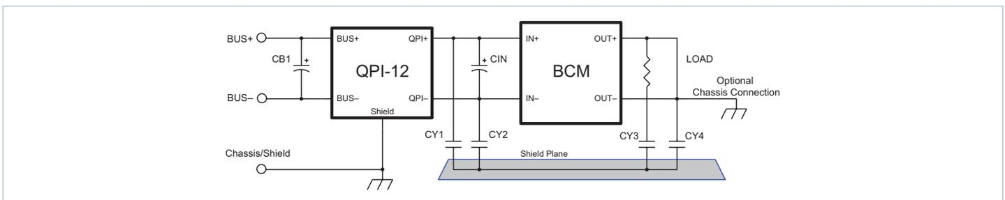
Typical QPI-12 application schematic with Vicor BCM module<sup>[a]</sup>
