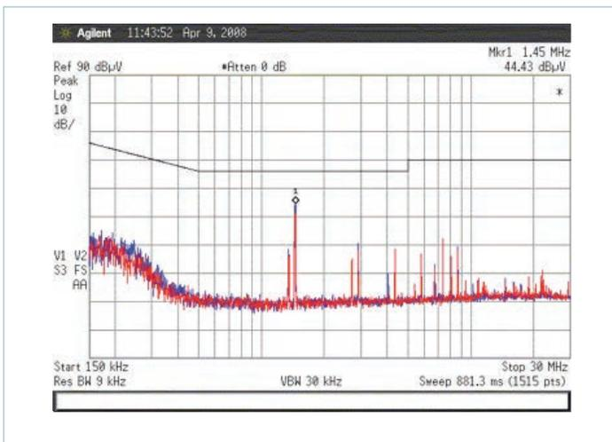
Figure 3 — VTM V048F030T070-CB with 160W load
