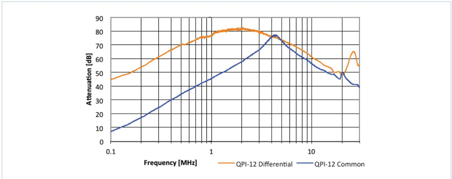
Figure 15 — Attenuation curves into a 50Ω line impedance, bias from a 48V bus
