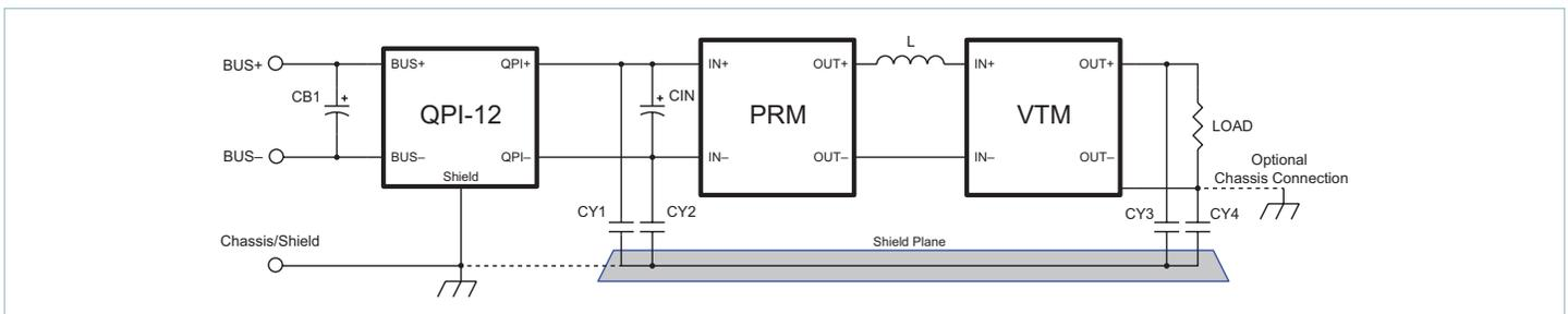
Typical QPI-12 application schematic with Vicor PRM and VTM modules<sup>[a]</sup>
