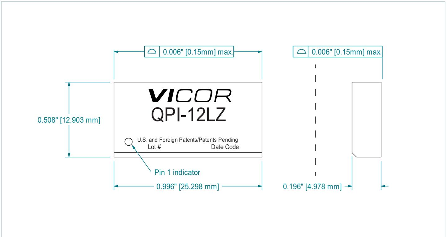
Figure 18 — Lidded package dimensions, tolerance of  $\pm 0.004$ in
