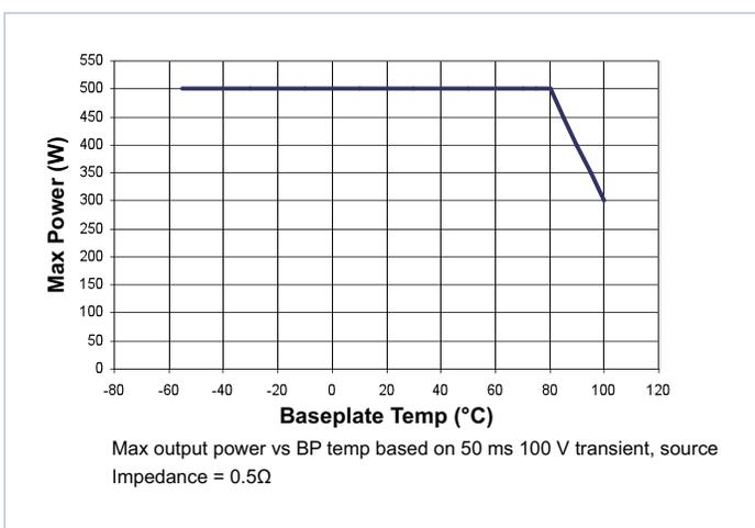
Figure 5 — Temperature de-rating
