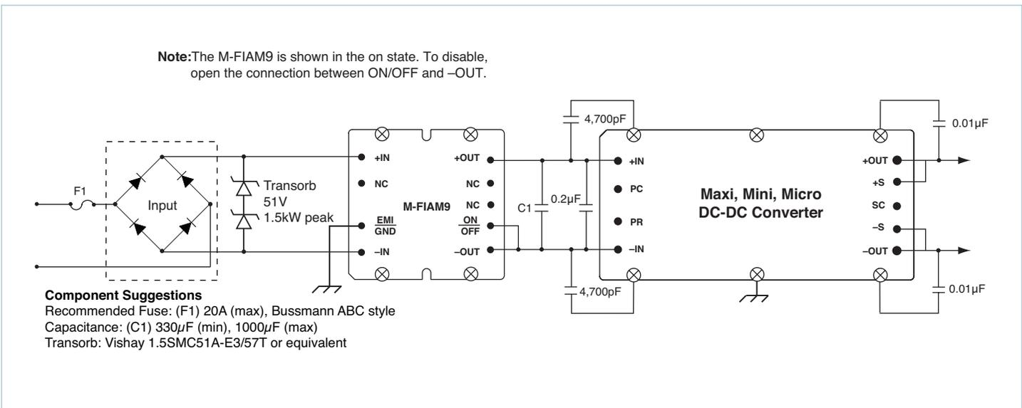
Figure 7 — Transient, surge protection and recommended reverse-polarity protection
