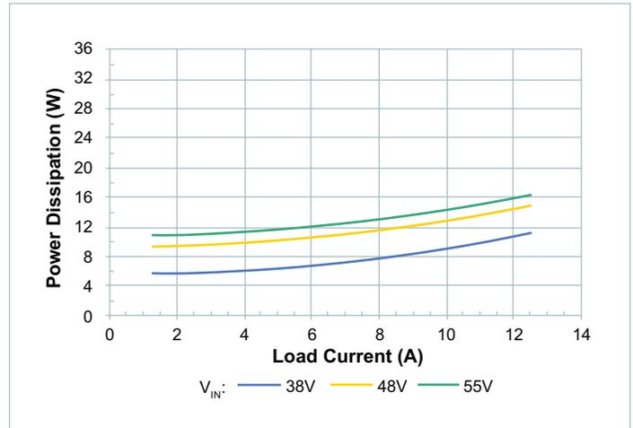
Figure 5 — Power dissipation at  $T_{CASE} = -40^{\circ}C$
