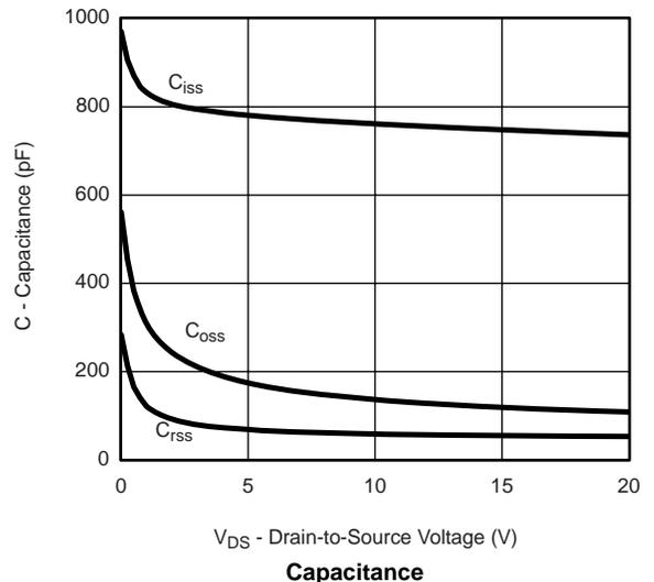
$V_{DS}$  - Drain-to-Source Voltage (V)
