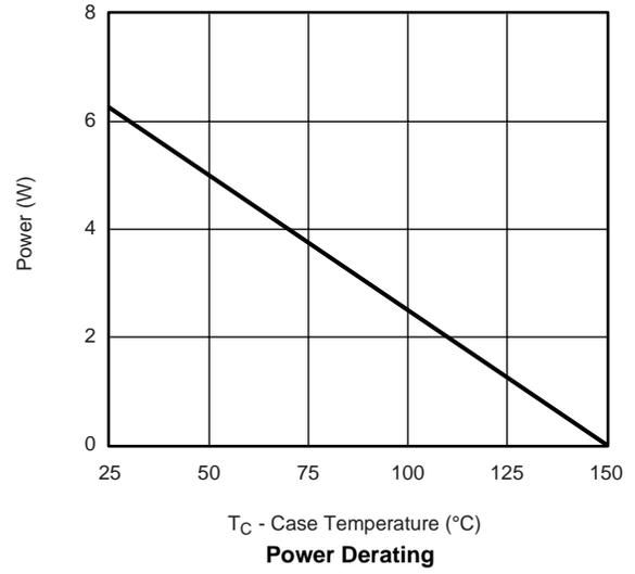
\* The power dissipation  $P_D$  is based on  $T_{J(max)} = 150\text{ °C}$ , using junction-to-case thermal resistance, and is more useful in settling the upper dissipation limit for cases where additional heatsinking is used. It is used to determine the current rating, when this rating falls below the package limit.
