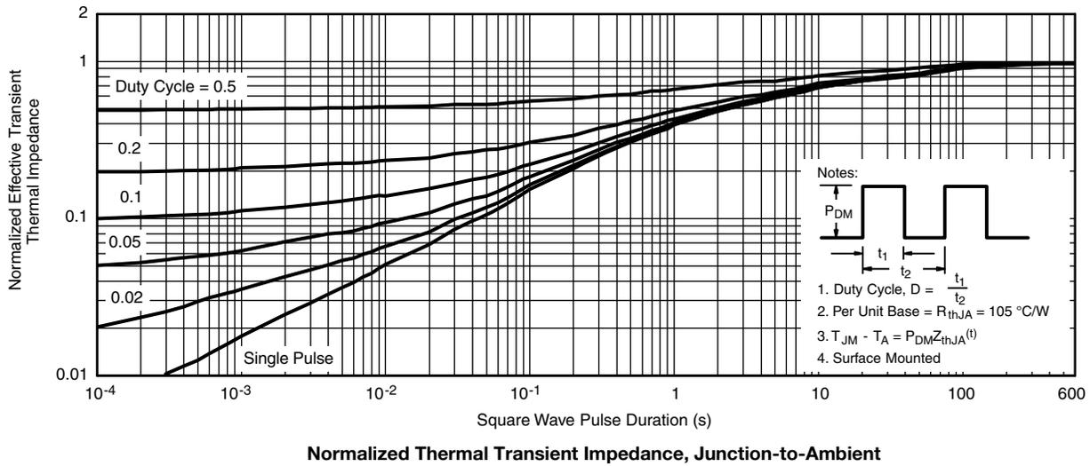
**THERMAL RATINGS** ( $T_A = 25\text{ }^\circ\text{C}$ , unless otherwise noted)
