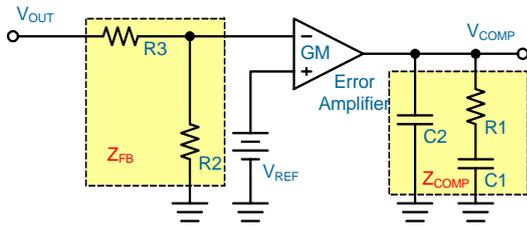
Figure 8. Type II Compensation Network Using OTA.
