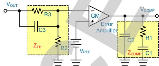
Figure 12. Type III Compensation Network.
