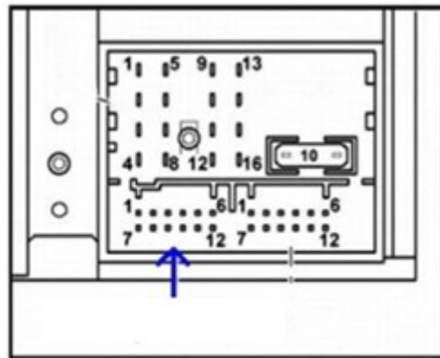
*Illustrative view of the back of the MFD radio to which you must connect the AUDIO adapter.*
