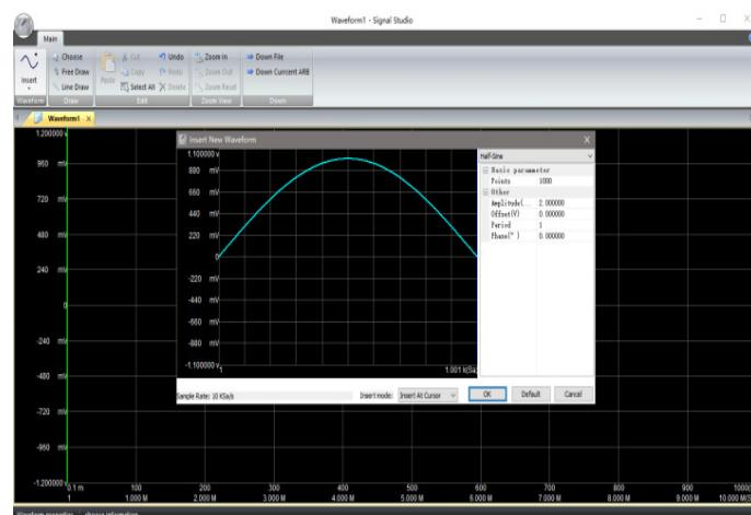
Generate arbitrary waveform through arbitrary waveform editor of upper computer.
