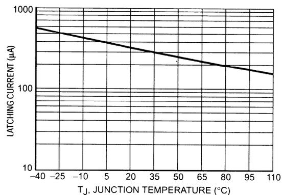
Figure 4. Typical Latching Current versus Junction Temperature
