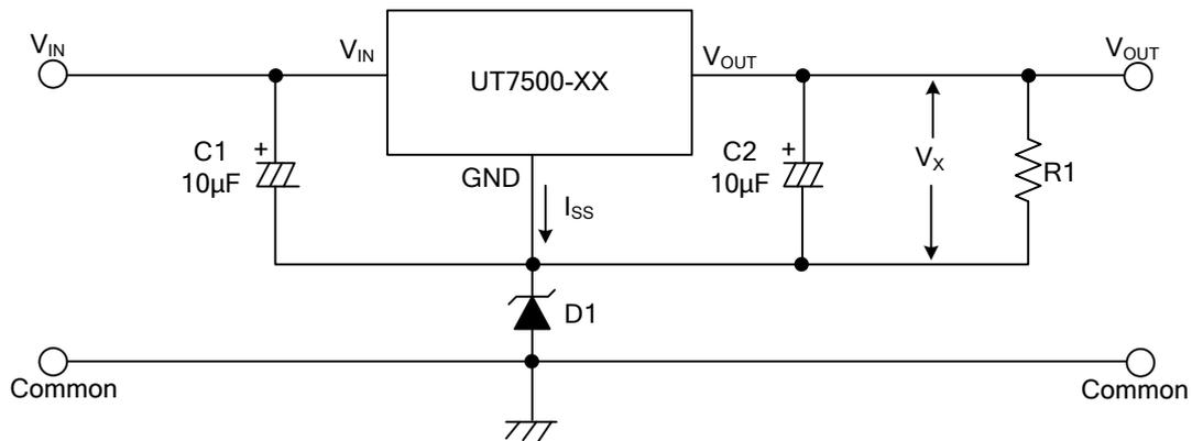
$$V_{OUT} = V_X + V_{D1}$$
