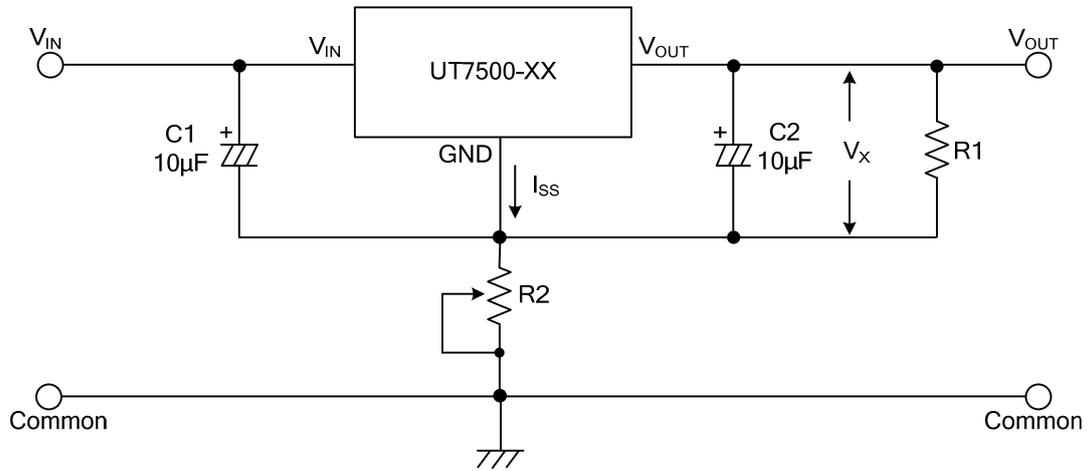
$$V_{OUT} = V_X (1 + R_2/R_1) + I_{SS}R_2$$
