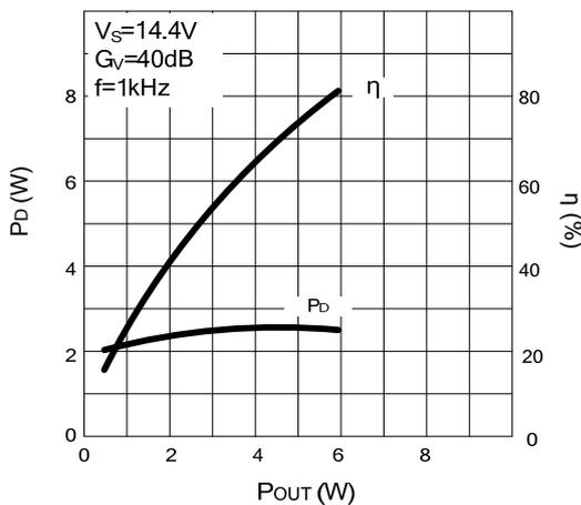
Power dissipation and efficiency vs. output power (R<sub>L</sub>=2Ω)
