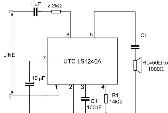
No current limitation is provided on the output stage of UTC **LS1240A**, so a minimum load DC of 50 ohms is advised.
