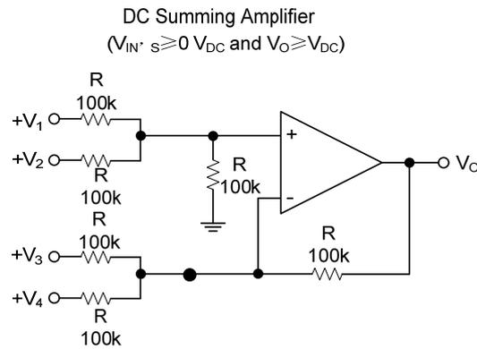
Where:  $V_0 = V_1 + V_2 - V_3 - V_4$ ,  $(V_1 + V_2) \geq (V_3 + V_4)$  to keep  $V_0 > 0 V_{DC}$
