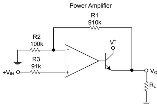
$V_0 = 0 V_{DC}$  for  $V_{IN} = 0 V_{DC}$ ,  $A_V = 10$
