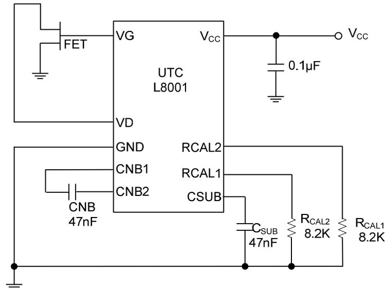
There are three major functions provided by L8001G: support negative voltage, bias control circuit, and FET protecting circuit.
