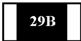
STANDARD E-96 VALUES AND 0603 RESISTANCE CODE
