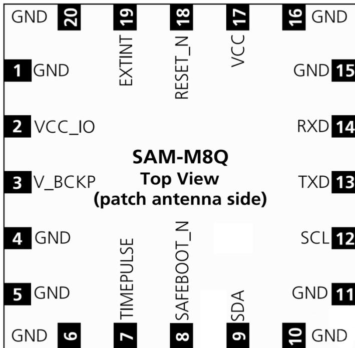
Figure 2: Pin Assignment
