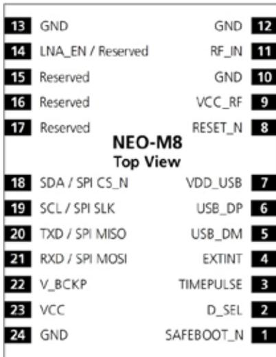
Figure 2: Pin Assignment
