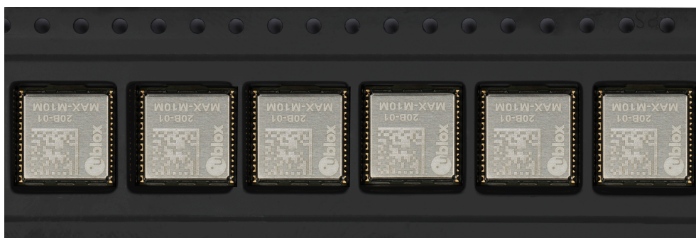
Figure 5: Orientation of the components on the tape
