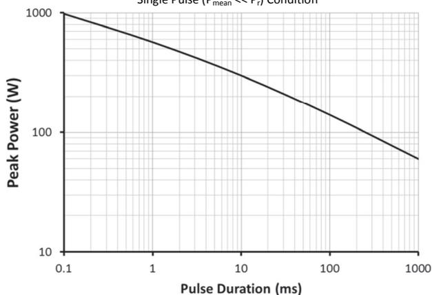
Pulse performance for durations ≥1s is dependent on mounting conditions. The short term overload power limit is 2 x power rating for 5s.
