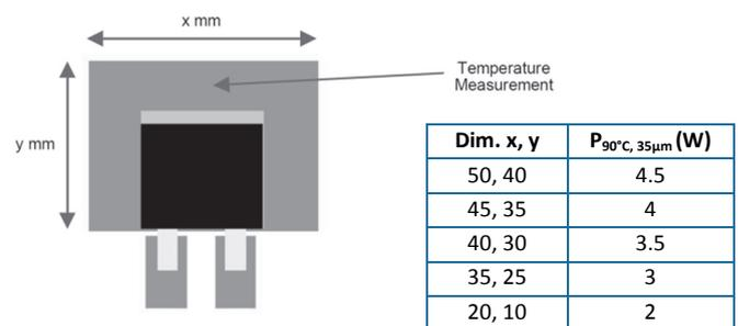
Characterisation carried out using 35μm PCB copper pad weights, with temperature of 90°C used as a maximum reference on the PCB. P<sub>90°C, 35μm</sub> (W) is power when the measurement point reaches 90°C.
