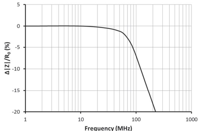
Typical high frequency characteristics for WSMHP35-220R. Self resonant frequency is 1GHz.
