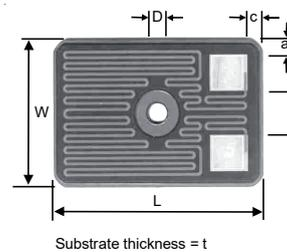
Fixing hole is located centrally except on WDBR1/2 where the dimension from the edge by the terminations to the mounting hole centre is 16.68mm.
