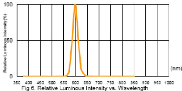
Fig.6. Relative Luminous Intensity vs. Wavelength
