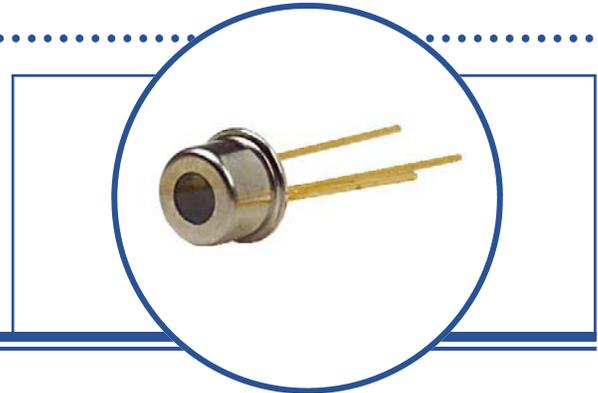
The OPF320 series fiber optic transmitters are high performance devices packaged for data communication links. This transmitter is an 850 nm GaAlAs LED and is specifically designed to efficiently launch optical power into fibers ranging in size from 50/125 $\mu$ m up to 200/300 $\mu$ m diameter fiber. Multiple power ranges with upper and lower limits are offered which allows the designer to select a device best suited for the application.
