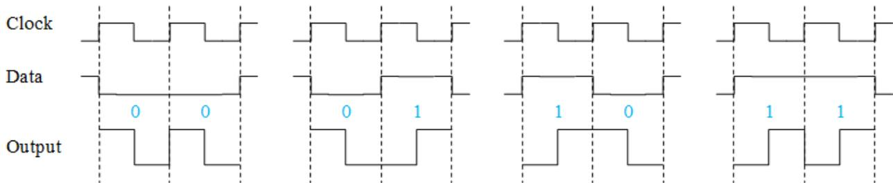
All commands sent to the OPB9000 are sent via the CAL/STAT pin. Each command must first begin with the syncing nibble (1100). The first two bits “11” allow the decoder to detect the data clock. The second two bits are a check for detection of the “00” data. The third two bits determine the command being sent. The available commands are:
