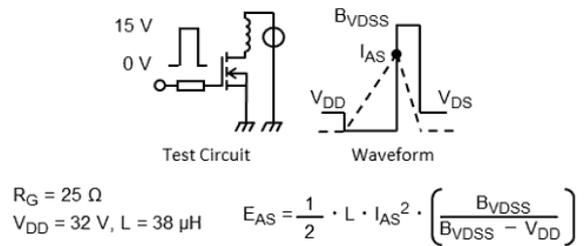
**Fig. 8.16 Test Circuit/Waveform**
