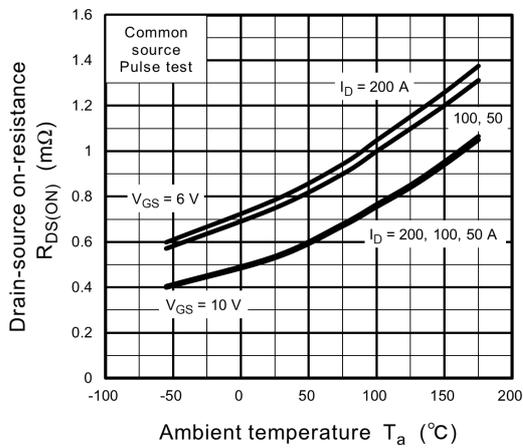
**Fig. 8.9  $R_{DS(ON)} - T_a$**
