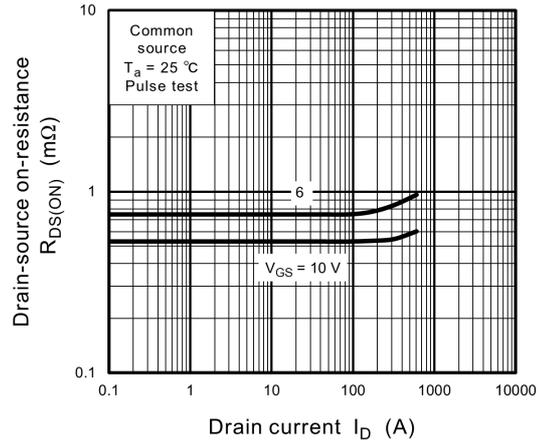
**Fig. 8.8  $R_{DS(ON)} - I_D$**
