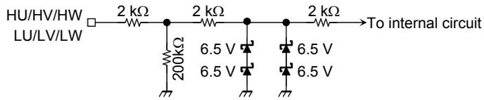
**Internal circuit diagram of RS pin**
