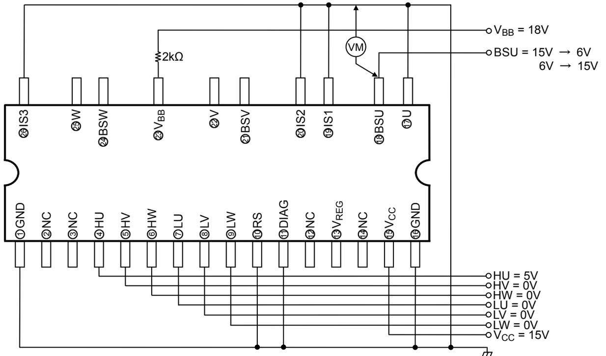
\*Note: Sweeps the BSU pin voltage from 15 V to decrease and monitors the VBB pin voltage. The BSU pin voltage when output is off defines the under voltage protection operating voltage. Also sweeps the BSU pin voltage from 6V to increase and change the HU pin voltage at 5 V→0 V→5 V each time. It repeats similarly output is on. When the BSU pin voltage when output is on defines the under voltage protection recovery voltage.
