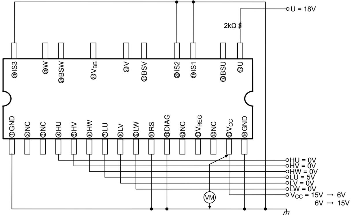
\*Note: Sweeps the VCC pin voltage from 15 V and monitors the U pin voltage. The VCC pin voltage when output is off defines the under-voltage protection operating voltage. Also sweeps from 6 V to increase. The VCC pin voltage when output is on defines the under voltage protection recovery voltage.
