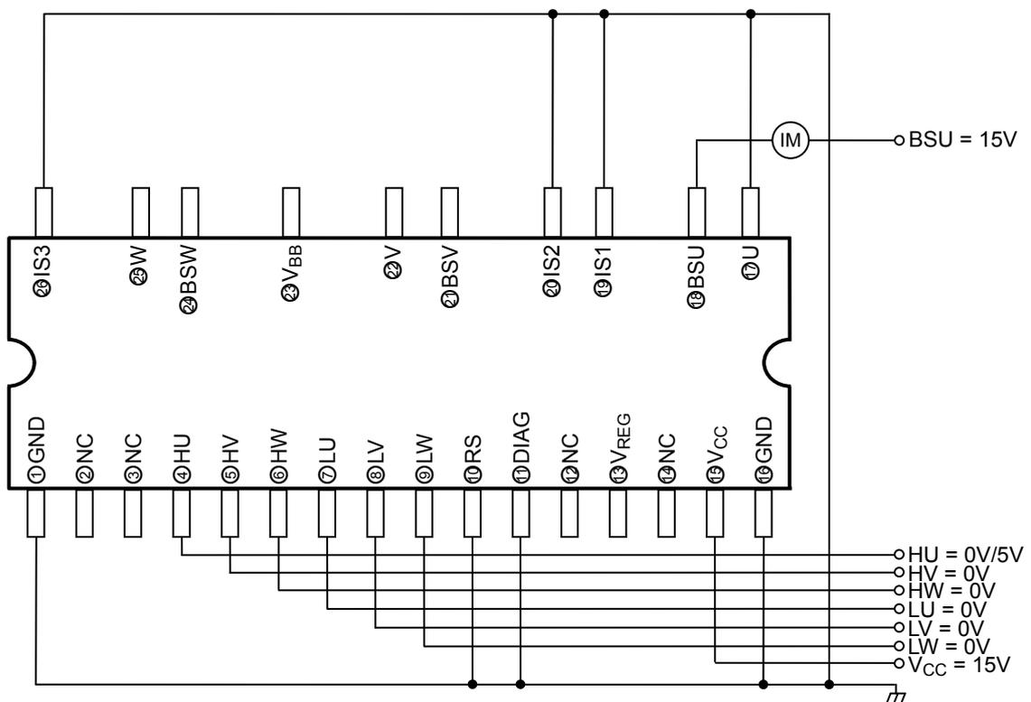
Turn-ON/OFF Loss (low side IGBT + high side FRD)
