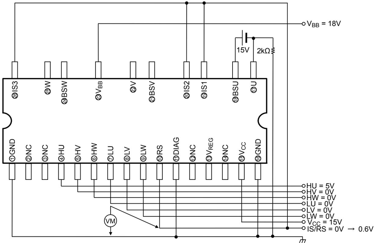
\*Note: Sweeps the IS/RS pin voltage and monitors the U pin voltage.
