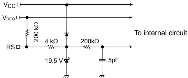
**Internal circuit diagram of DIAG pin**
