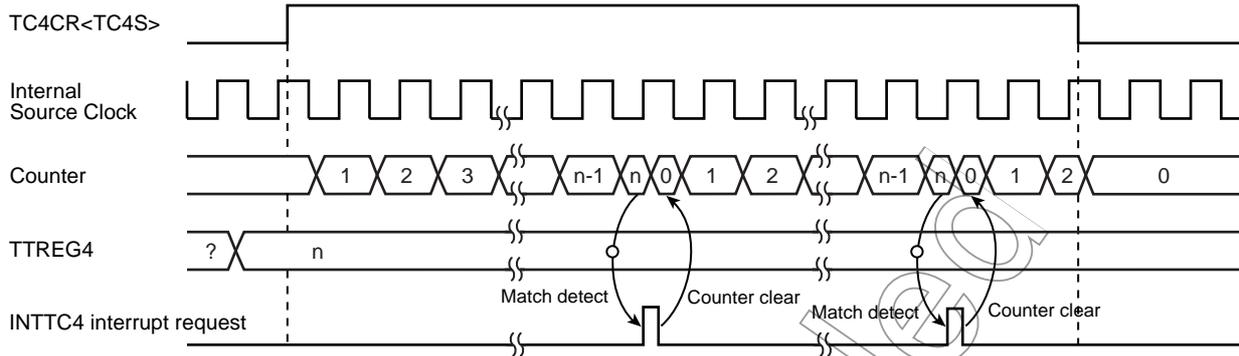
Figure 9-2 8-Bit Timer Mode Timing Chart (TC4)
