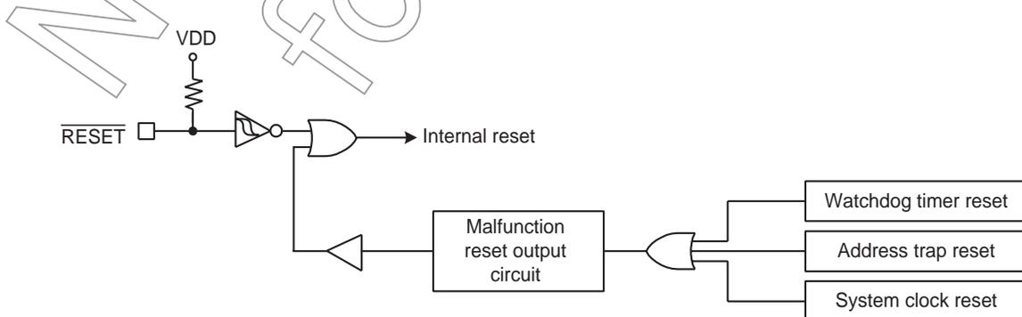
Figure 2-15 Reset Circuit
