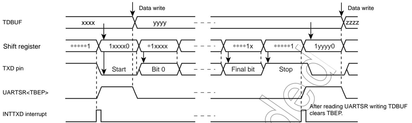
Figure 10-9 Generation of Transmit Data Buffer Empty
