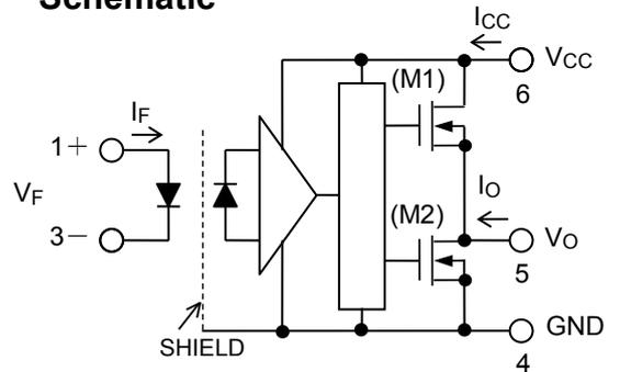
Note: A 0.1- $\mu\text{F}$  bypass capacitor must be connected between pins 6 and 4.
