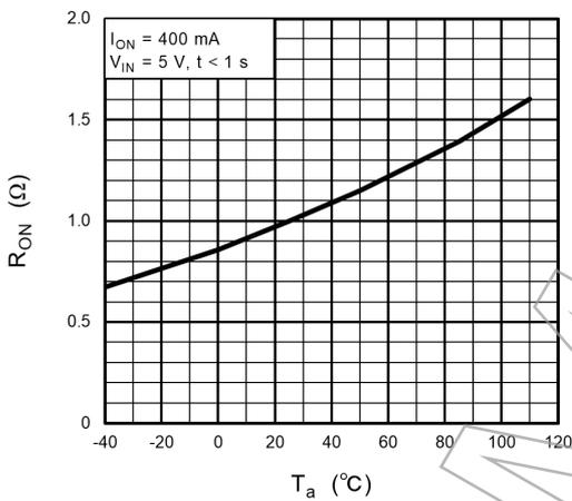
Fig. 12.3  $R_{ON} - T_a$
