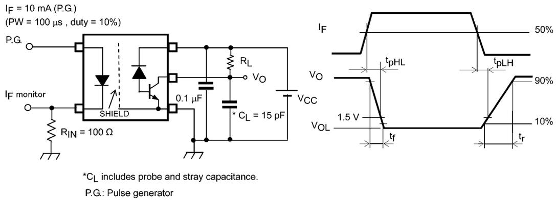
Fig. 12.1.1 Switching Time Test Circuit and Waveform
