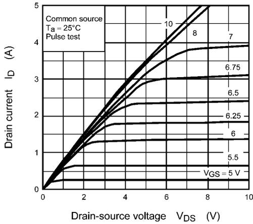
**Fig. 8.1  $I_D - V_{DS}$**
