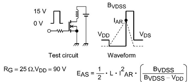
Fig. 8.16 Test Circuit/Waveform
