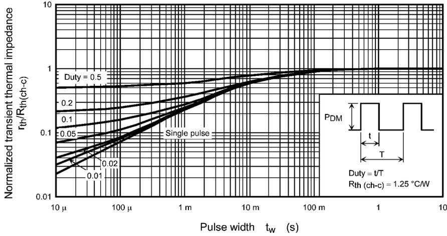
Fig. 8.13  $r_{th}/R_{th(ch-c)} - t_w$
