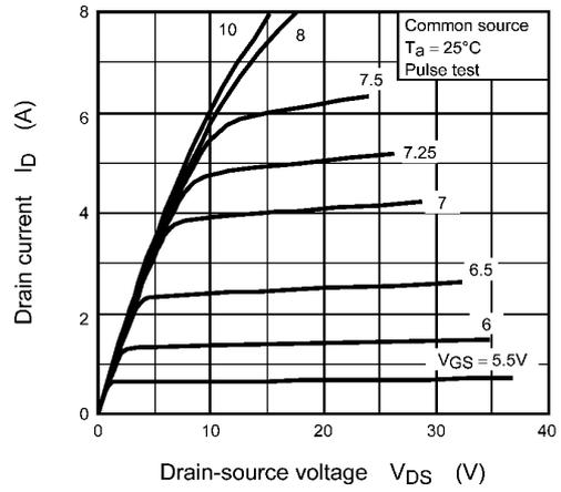
**Fig. 8.2  $I_D - V_{DS}$**
