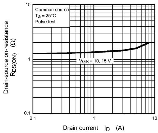
**Fig. 8.6  $R_{DS(ON)} - I_D$**
