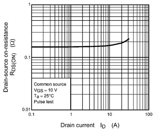
**Fig. 8.6  $R_{DS(ON)} - I_D$**
