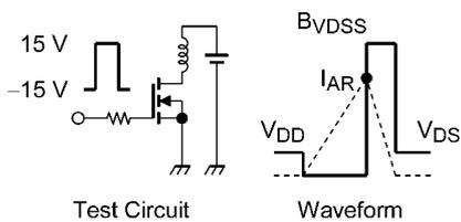
$R_G = 25 \Omega, V_{DD} = 90 \text{ V}$   $E_{AS} = \frac{1}{2} \cdot L \cdot I_{AR}^2 \cdot \left( \frac{B_{VDSS}}{B_{VDSS} - V_{DD}} \right)$
