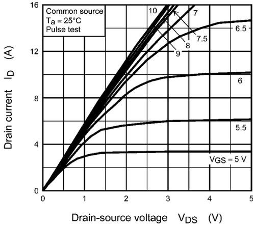
**Fig. 8.1  $I_D - V_{DS}$**
