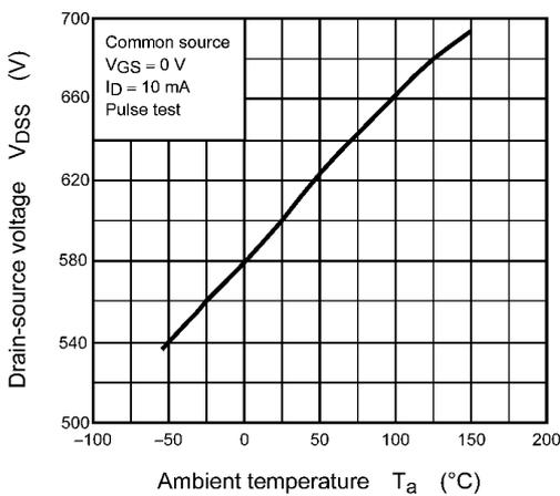
**Fig. 8.5  $V_{DSS} - T_a$**
