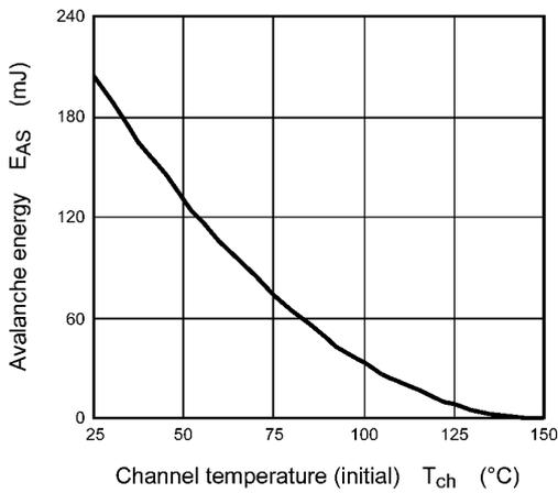
**Fig. 8.14  $E_{AS} - T_{ch}$**
