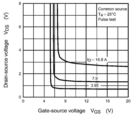
**Fig. 8.4  $V_{DS} - V_{GS}$**
