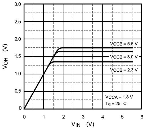
Fig. 15.2 Input/Output Characteristics (Typ.)
