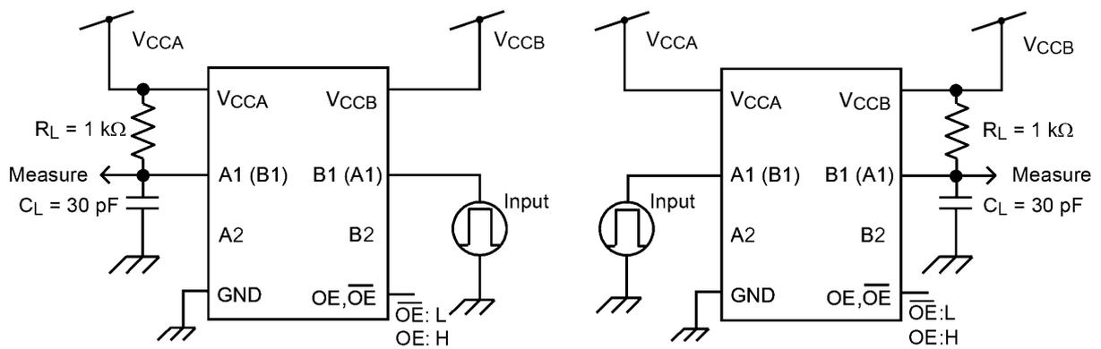
Fig. 13.1  $t_{PLH}$ ,  $t_{PHL}$  Test Circuits
