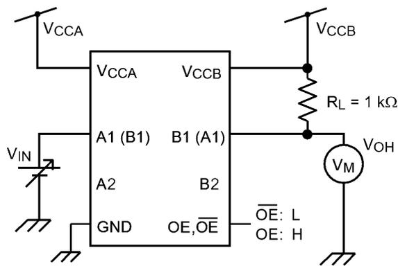
Fig. 14.1 Test Circuit
