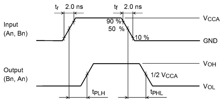
Fig. 13.3 AC Waveform of  $t_{PLH}$ ,  $t_{PHL}$
