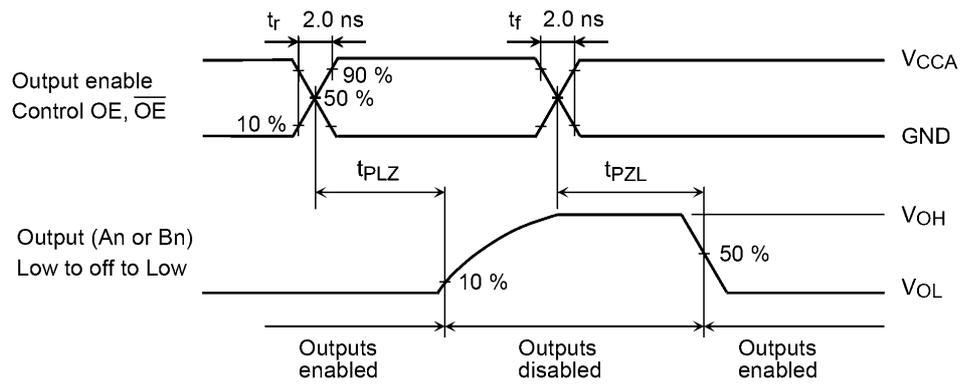
Fig. 13.4 AC Waveform of  $t_{PLZ}$ ,  $t_{PZL}$
