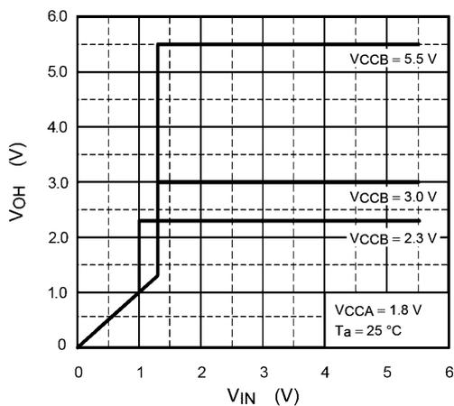
Fig. 14.2 Input/Output Characteristics (Typ.)
