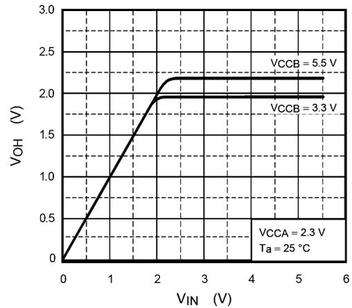
Fig. 15.3 Input/Output Characteristics (Typ.)
