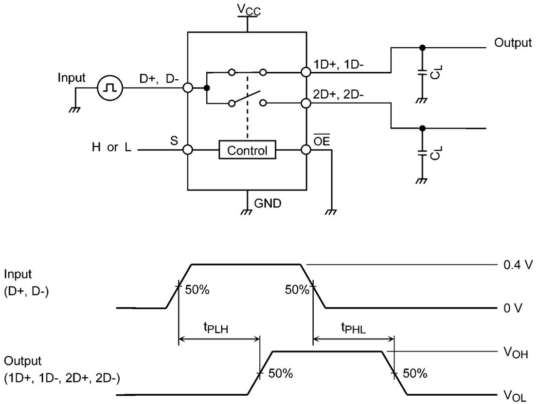
Fig. 11.1 Propagation Delay Time ( $t_{PLH}$ ,  $t_{PHL}$ )
