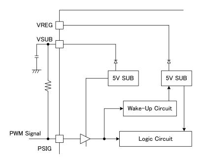
Note: Please do not use the 5V SUB regulator (VSUB) as a power supply (Hall device supply, others) of an external element.
