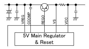
The over current detection circuit is a circuit that detects the current flowing in the 5 V power supply circuit with the external resistor R, and turns off the REGO pin when the voltage drops more than Vlimit so that the current does not flow more than a certain amount.
